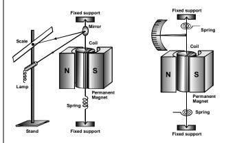
WORKING: When current "I" is passed through the coil, the coil is acted upon by a couple, called deflecting couple, which tends to rotate the coil. The deflecting torque is given by:
